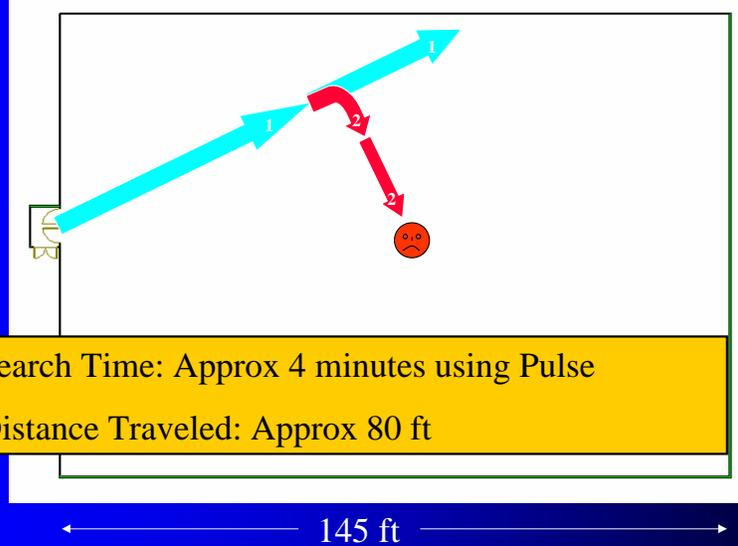
For this test, the rescue team was told that there a firefighter had fallen through the roof near the center of the building. A Beacon in muted alarm mode (that is, ultrasound on, audible sound off) was placed on the victim. The team headed into the building, thinking they were headed towards the center of the room. In fact, they were about 30 degrees to the left. The team leader headed into the building and the firefighter #2 had a Tracker.
