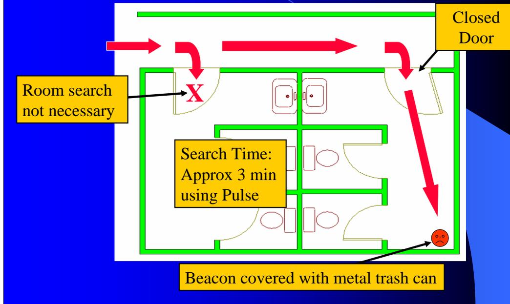
Because the previous search using the Pulse System was essentially a direct line to the victim, one instructor decided to give the system a more-difficult test. He said he would hide the Beacon and see if the second instructor could find it. The Beacon was put into muted alarm mode (ultrasound on, audible sound off).
