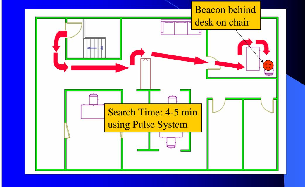
In this evolution, a Pulse Beacon was placed on a chair behind the desk in the same small office as the previous blind search. The Beacon was placed into muted alarm mode (that is, ultrasound on, but audible sound off).
